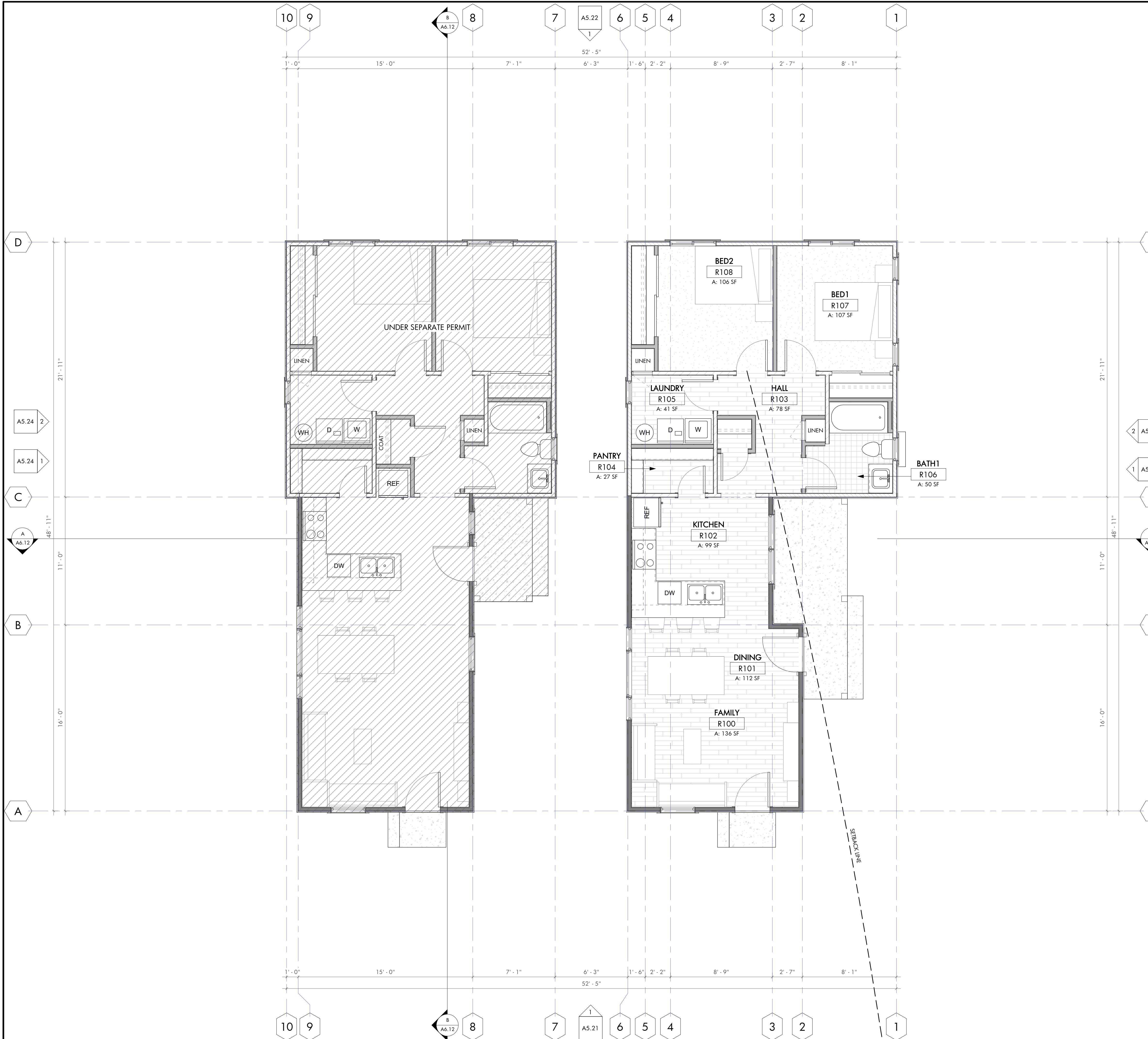
114 LEVEL-1 FLOOR PLAN 1/4" = 1'-0"
